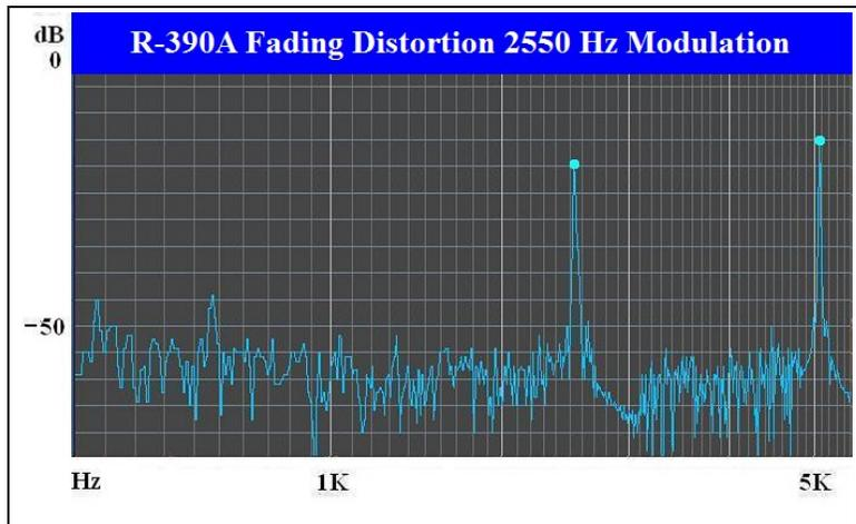
Note that the fading distortion for the WJ-8711A (in the figure at right) is about the same as for the R-390A (above). Also note the spurious DSP distortion 10 dB below the fundamental and 18 dB below the 2nd harmonic. Such distortion has not been observed in analog receivers.
