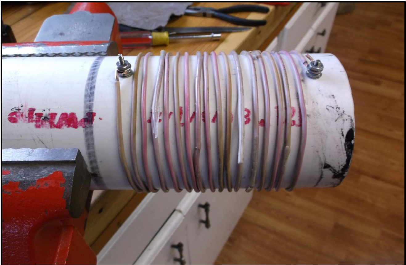
Figure 2 - Old radial wire wound into an inductor.
