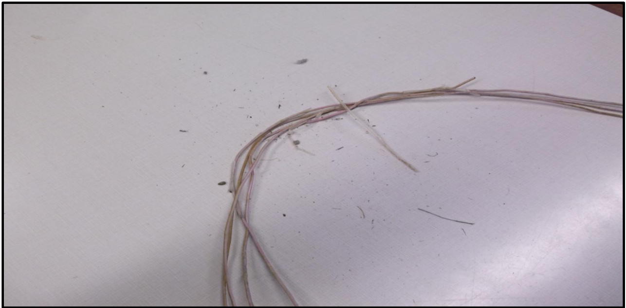
Figure 1 - Sample of degraded #12 radial wire.
