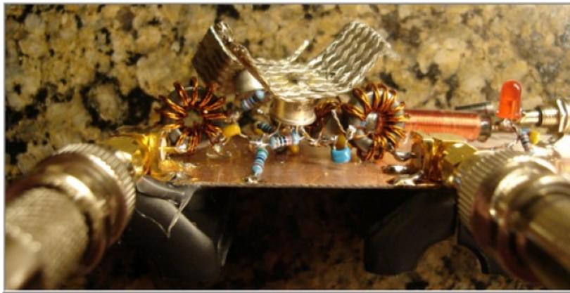
Voltage references: Vb-gnd 5.6v, Ve-gnd 4.88v
