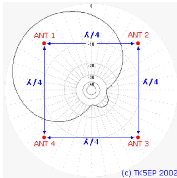
**Azimuth and position of antennas, system in NW position.**
