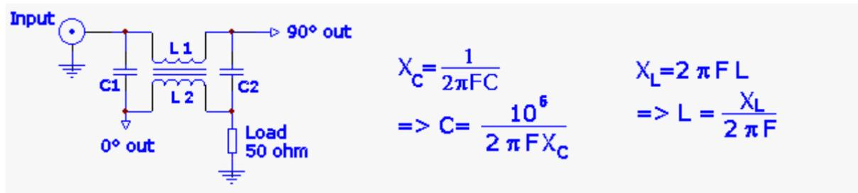
Where  $X_c = 100 \text{ ohm}$ ,  $X_L = 50 \text{ ohm}$ ,  $L$  in  $\mu\text{H}$ ,  $C$  in  $\text{pF}$ ,  $F$  in  $\text{MHz}$ ,  $C1=C2$  and  $L1=L2$
